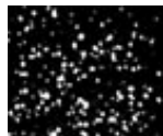
Charged air-assisted spray on leaf underside. Average count in 54 samples = 425 deposits in 1/8 in 2
